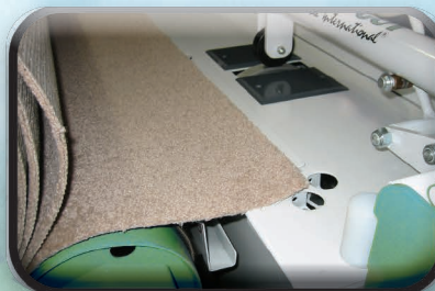
AUTOMATICALLY KEEPS THE ROLLS STRAIGHT WITH PHOTO-SENSOR EYES
